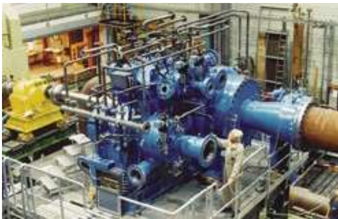
FIG. 4 Type RG 80-8 8-stage integrally geared compressor (CO 2 ) for gas injection.
