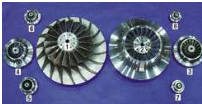
FIG. 5 High-pressure CO 2 integrally geared compressor impellers.
