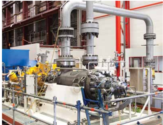
Main oil pump (~100,000 bpd) on test bed (courtesy of Flowserve).
